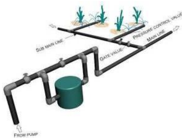
FIGURE 10. The sprinkler irrigation system
